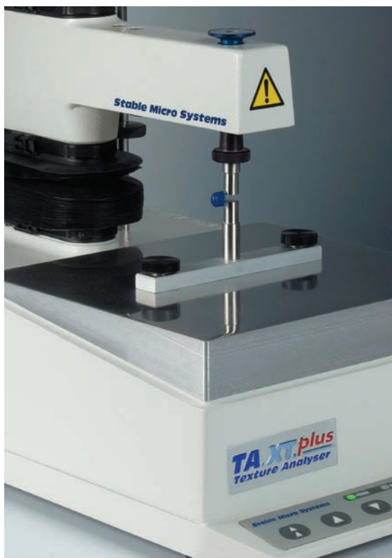
The Capsule Tensile Rig measures strength and stability of hard gel capsules, enabling manufacturers to identify the effects of fillings on the mechanical strength of the capsule shell.
